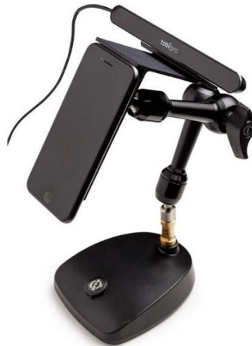
Fig. 2. Using Tobii Pro Nano with a smartphone [21]
