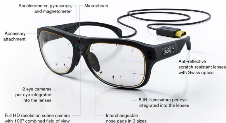
Fig. 3. Structure of Tobii Pro Glasses 3 [22]
