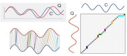
Figure 3. (a) Time series C and Q and the linked points in time by DTW. (b) Minimum warping path W through the LCM of time series C and Q.
