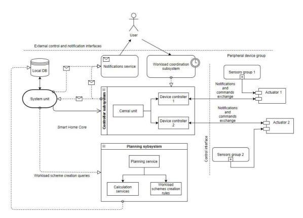
Figure 1. Hierarchical components structure scheme
